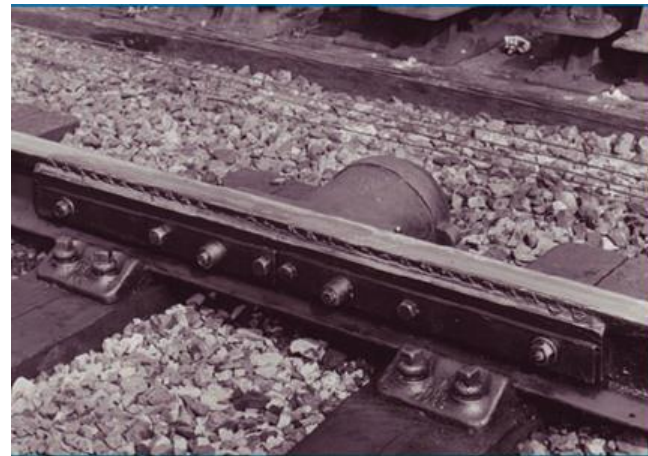
P&M Model C4L Mechanical Lubricator installed on British Rail in the UK, circa 1953
